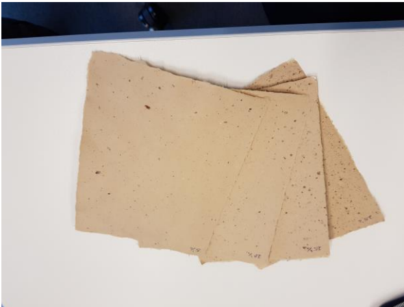
Papersheets made with different cocoashell loadings (Schut Paper)
