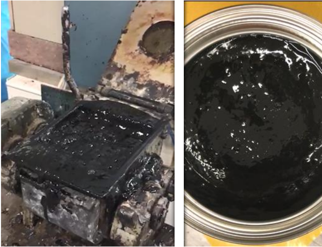
Preparation of a lignin-bitumen blend for carpet tile backing (Interface)
